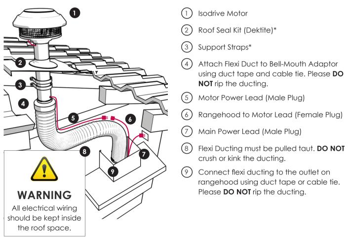
\***NOTE:** The Isodrive motor system does not include the roof seal kit, cable tie, duct tape or the support straps. The weather shield is only available for the Isodrive 1600 motor and needs to be attached directly to the motor (1).
