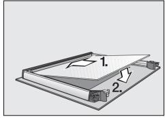
■ Refit the middle pane in such a way that the material number is legible (i.e. not reversed).
