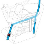
Rear facing seatbelt lockoff. Sash belt side clamps lap belt portion only
