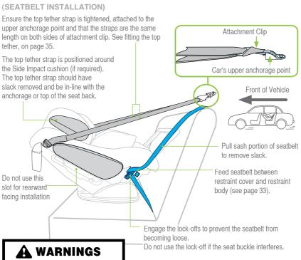
DO NOT USE RESTRAINT IN REARWARD FACING MODE WITHOUT STABILISING BAR FULLY EXTENDED. THE TOP TETHER STRAP MUST ALWAYS BE FITTED WHEN THE CHILD RESTRAINT IS USED IN A VEHICLE. ALWAYS ATTACH THE HOOK AND REMOVE THE SLACK.
