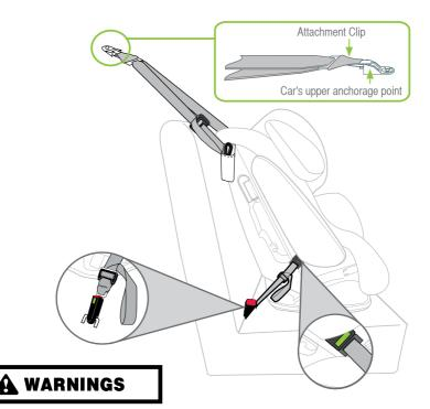
DO NOT USE RESTRAINT IN REARWARD FACING MODE WITHOUT STABILISING BAR FULLY EXTENDED. THE TOP TETHER STRAP MUST ALWAYS BE FITTED WHEN THE CHILD RESTRAINT IS USED IN A VEHICLE. ALWAYS ATTACH THE HOOK AND REMOVE THE SLACK.
