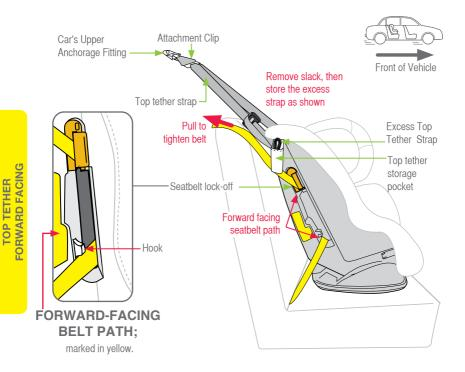
IMPORTANT: THIS RESTRAINT IS NOT SUITABLE FOR USE WHERE THE TOP TETHER STRAP MAY FALL INTO A SPLIT IN THE SEAT BACK OR OFF THE SIDE OF THE SEAT.
