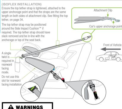
DO NOT USE RESTRAINT IN REARWARD FACING MODE WITHOUT STABILISING BAR FULLY EXTENDED. THE TOP TETHER STRAP MUST ALWAYS BE FITTED WHEN THE CHILD RESTRAINT IS USED IN A VEHICLE. ALWAYS ATTACH THE HOOK AND REMOVE THE SLACK.
