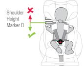
Turn to forward-facing when the child's shoulders are between the lower marker A and middle marker B shoulder height markers.
