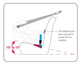
Illustration shows child seat installed with seatbelt. Also applicable to an ISOFLEX installed variant.
