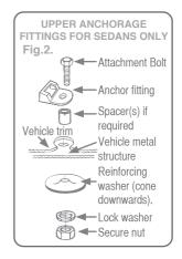
ONLY USE A 5/16 UNC GRADE 5 BOLT. IF THE BOLT IS NOT THE CORRECT LENGTH THE CAR MANUFACTURER'S HAND BOOK CAN PROVIDE ADVICE ON THE CORRECT LENGTH BOLT.
