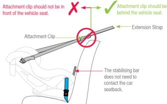
It is normal to have some sideways movement if the headrest end is pushed from the side. Ensure that the seatbelt is tight and the slack is removed from the tether strap. If the tether strap is over tightened, the angle of the child seat may be affected.
