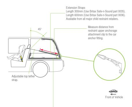
The shaded areas of this diagram illustrate the possible locations of the upper anchorage point (car anchor fitting). Within each shaded area is an upper anchorage point showing the correct way to install the fitting. Ensure the upper anchorage point is aligned as illustrated unless stated otherwise in the vehicle owner's handbook.
