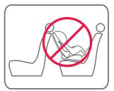
Do not allow the front seat to alter the installed angle of the restraint. It is permissible to allow the restraint to touch the front vehicle seat.
