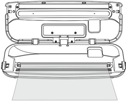
4. Close and lock lid by pushing the silver arrows on each side of the lid until fully closed.
