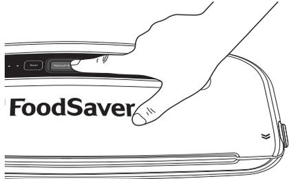
6. After the sealing light has gone out, press the 2 release buttons on either side of the appliance to release the lid and remove bag.
