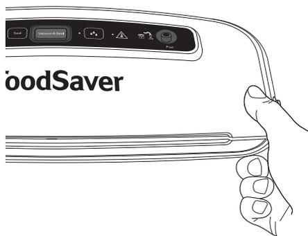
7. Press the seal button. When the seal indicator light turns off, open the lid by pressing the 2 release buttons on either side of the appliance. Remove the bag.
