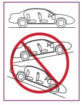
Position base on a forward facing vehicle seat. Use recline adjustment to position bubble in indicator.
