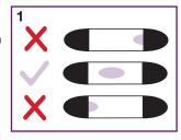
2 Use recline adjustment, if needed, to achieve correct angle for installation. Recline adjustment foot snaps into position.
