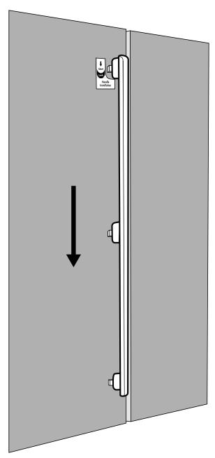
Note: After fitting the handle give a gentle tug in an upwards direction to confirm the handle is fully located. Once fully located the handle can not be subsequently removed.
