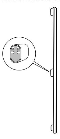
**Step 2.**Position handle over handle mounts and align with
