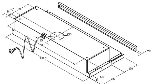
The maximum space between the wall and screw cap is 5mm.
