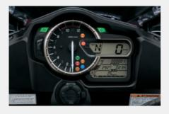
The instruments include an analogue tachometer and a brightness-adjustable LCD speedometer. LCD readouts include an odometer, dual trip meters, the gear position, the coolant and ambient temperatures, the voltage, the riding range, the average fuel consumption, the instantaneous fuel consumption, the traction control mode, a fuel gauge, and a clock...
