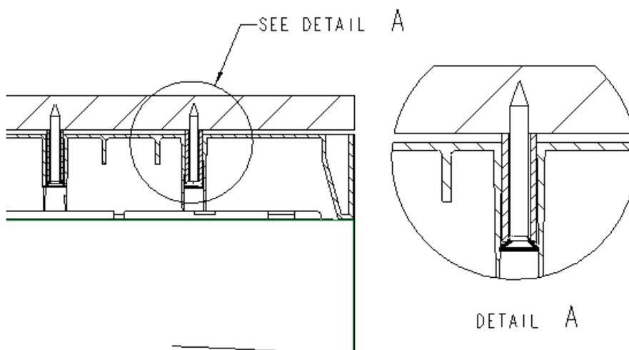
**PLEASE NOTE:** Using the incorrect screws for the installed mounting method or not using the metal tubes as per these instructions may cause damage to the product. This damage may lead to failure of the side mounting anchor points and this would not be covered by the warranty.
