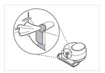
3 Clean the cliff detection sensors ① and the charging terminals ② of the Robot Cleaner using a cotton swab or a soft cloth.
