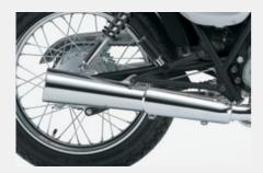
Exhaust system is outfitted with a catalytic converter and oxygen sensor feedback system reducing exhaust emission.
