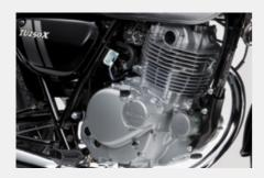
249cc four-stroke single-cylinder engine features a simple, lightweight, air-cooled SOHC design with class-leading Suzuki fuel injection, and produces strong low-RPM torque, which makes the TU250X a perfect choice for the city rider.
