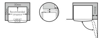
NOTE: Refrigerator doors on all models are designed to sit proud of cabinetry (not flush). The refrigerator should be placed against a wall of cabinetry and the clearance between the rear of the refrigerator and the wall should not be greater than 75mm.
