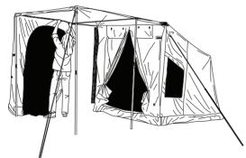
Fully extend the 2.2m Awning Poles when the Peaked Side Panel is zipped on half way.
