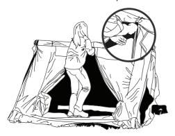
**5** Reach inside the tent and velcro the internal frames to lock in place.
