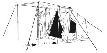
Assemble your ridge pole. Twist to lock at desired location.
