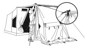
Peg at all base peg points and set up support poles. Extend all guy ropes, peg and secure.
