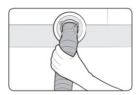
2. Insert the drain hose into the drain outlet. Make sure to connect them firmly using the joint ring. The drain hose is extensible. Adjust the length of the drain hose as needed.
