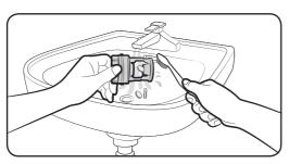
**1.** Put a floor-cloth or towel under the Pump filter. Turn the filter knob anticlockwise to remove.
