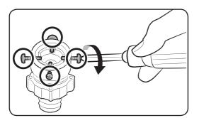
**2.** Use a Philips screwdriver to loosen four screws on the adaptor.
