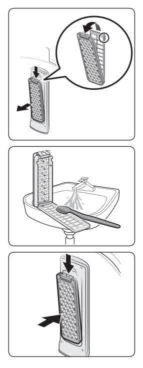
**1.** Press down the upper area of the filter case to remove.
