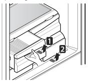
To install, slightly tilt up the front, insert the drawer into the frame and push it back into place.
