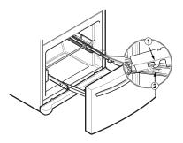
3 Lower door into final position and tighten the screws ③. Make sure you have a right rail cover for each side.
