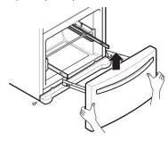
5 With both hands, flex the center bar enough to allow the gears on both ends to release from the track.
