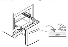
3 Remove the screws of the rail on both sides.
