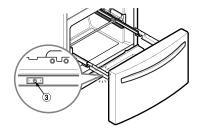
4 Align the top holes of the rail cover with the top holes of the door supports to assemble the rail covers.
