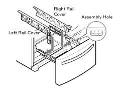
5 With the drawer pulled out to full extension, insert the lower basket in the rail assembly.
