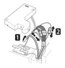
4 Rotate the hinge lever counterclockwise
