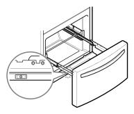
4 With both hands, hold both sides of the door and pull it up to separate it from the rails.
