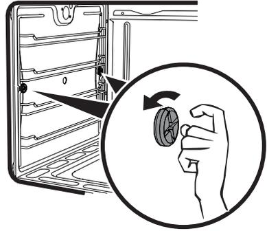
2. pull out the frame toward the interior. If self-cleaning panels are fitted they have to be removed together with the frame.
