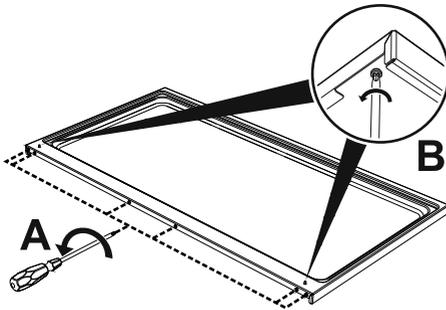
2. Place the backguard on the top. Align the 6 bottom slots of the backguard with the 6 screws on the back of the top that were previously loosened.
