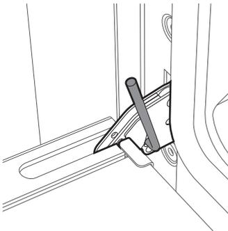
2. Grasp the door on both sides with both hands, lift it forming an angle of around 30° and remove it.
