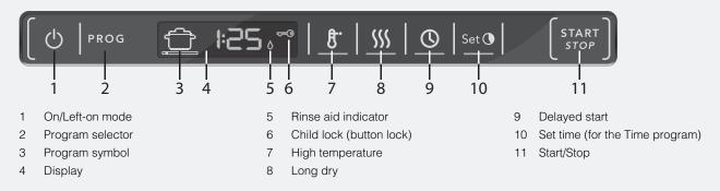
The panel is fitted with touch buttons with audible feedback (see the chapter Settings).
