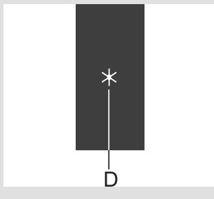
To activate the freezer boost function, press the **B** key until the symbol **D** lights up.
