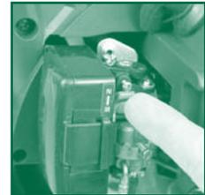
2. If the engine is cold, move the choke (15) lever upwards
