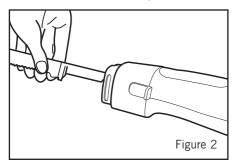
3. Insert the plug into a 230-240 volt (AC only) power outlet and ensure the cord is well away from the blades. Holding the knife with one hand, slide and press the power trigger positioned under the handle to activate the motor. Releasing the switch will automatically stop the motor.
